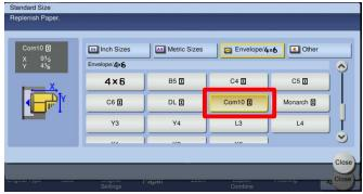
\*NOTE: Large and odd size envelopes can also be run in Tray 1 and would need to be set up as "Custom Size". They can also be done in the BYPASS TRAY (\*maximum 10 envelopes in Bypass Tray).
